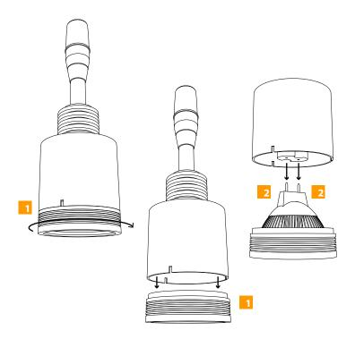
Insert a small hex key, push pin, or paper clip into one hole in the lamp retaining ring and twist counter clockwise to unscrew
